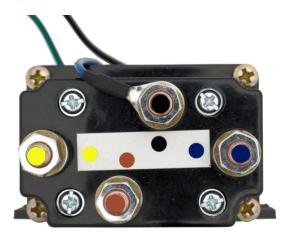
Connect BLUE post to the winch BLUE post Connect YELLOW post to the winch YELLOW post Connect RED post to the battery POSITIVE post Connect BLACK post to the battery NEGATIVE post
